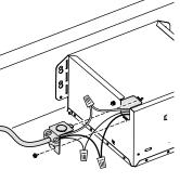
details. Use screw (from parts bag) to secure wiring plate to fan housing. Re-install wiring panel and secure with screw from parts bag.
