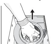
Remove wiring panel from fan housing (if already installed).
