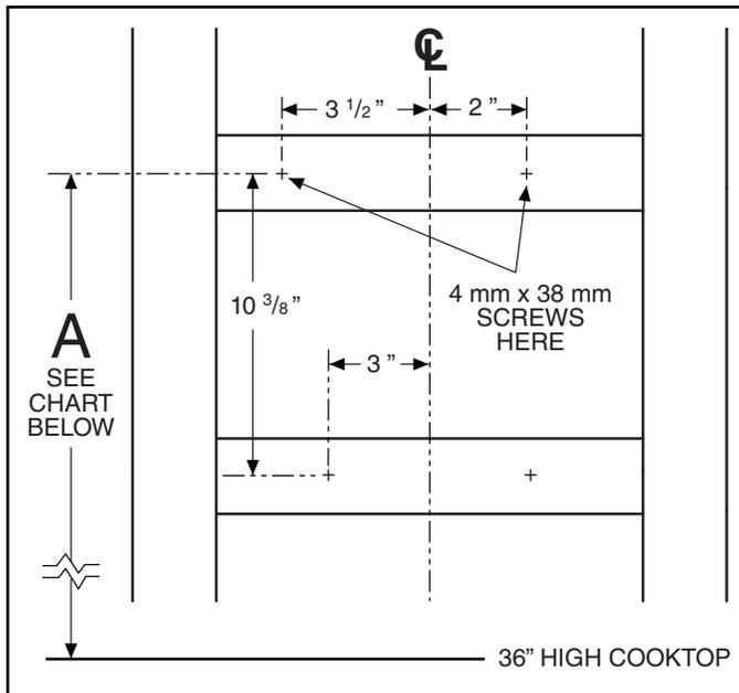
1. Construct wood wall framing that is flush with interior surface of wall studs. Make sure the framing is centered over installation location.
