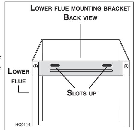
Both lower and upper flues are included with the hood, but for a 10-foot ceiling, discard the provided upper flue and use the optional flue extension, part no. FXN58SS (sold separately).
