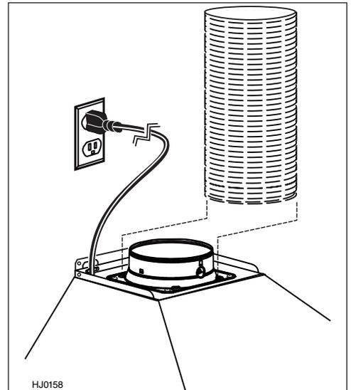
Using 4 ST4 x 8 provided screws, assemble the 6" round adapter to the plenum.
