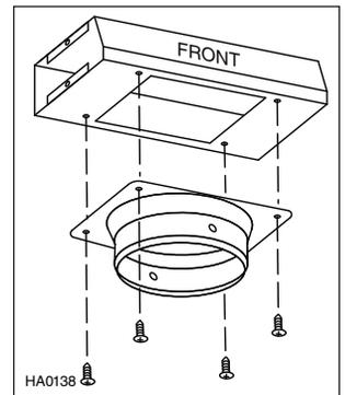
Attach the aluminum flexible duct to the non-duct plenum collar. Make sure non-duct plenum "FRONT" is facing front of hood. Secure with tie wrap and seal with metal foil duct tape.
