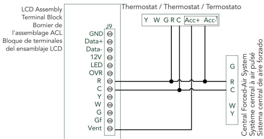
1 - External switch or any dry contact can be used to activate Vent input if not available on the thermostat
