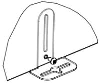
**IMPORTANT:** Fully insert the brackets in the unit to align both holes (not the slot). Use short screws provided to secure it.
