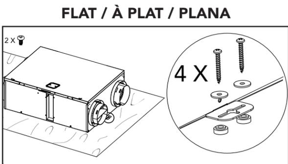
**NOTE:** To prevent vibration transmission, do not overtighten or deform dampening washer.
