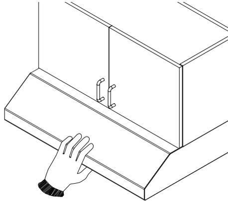
WHILE HOLDING THE HOOD, secure the hood to the cabinet using 4 round head wood screws (included in parts bag). Use 2 screws per side.
