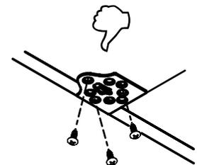
Outer side of the bracket flush with hood side.
