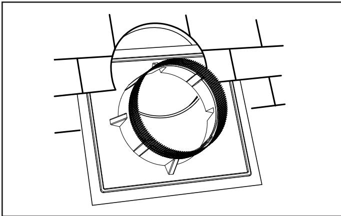
12. Apply a large bead of roofing cement in the molded groove on the bottom side of ventilator base. Make sure the arrow on the ventilator base is pointed toward the roof ridge. Start two-thirds of the way down from the top of the 27" square and slide the ventilator base under the shingles. Do not bend the shingles any more than necessary. Center the ventilator base over the hole.
