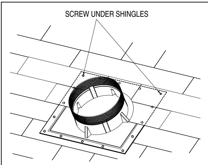
13. Make sure the ventilator base is parallel to the roof ridge, carefully lift shingles and screw base securely to the roof using galvanized #10 x 1" pancake head wood screws. Screw all corners and around perimeter of base every 6 inches.
