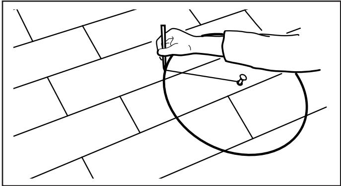
6. From the roof side, using the guide hole as the center point, use a nail and string to scribe a 16-1/2" diameter circle on the shingles. Note: If replacing an existing ventilator, the hole diameter may be larger than 16-1/2". This is acceptable provided the roofing material overlaps the ventilator by at least 2" on all sides.
