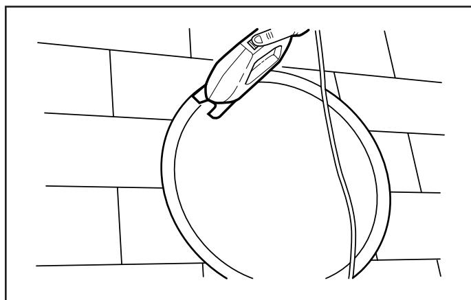
10. Cut out the roof board(s) inside of the line.
