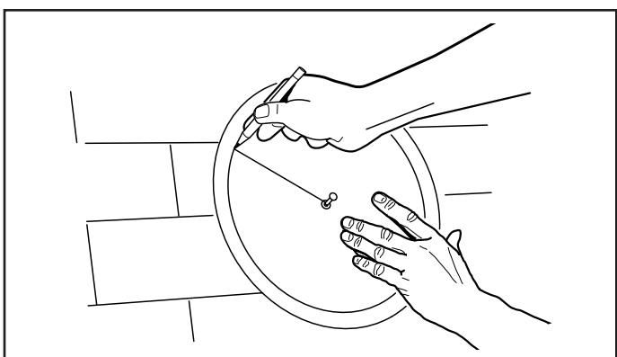
8. Using the same nail and string shown in step 6, scribe a 14" diameter circle on the black paper or roof decking. Note: if replacing an existing ventilator the hole diameter may be larger than 14". This is acceptable provided the ventilator base is adequately supported by the roof decking.
