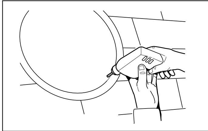
9. Drill a large starting hole for the sabre saw just inside of the line or the 14" circle created in Step 8.
