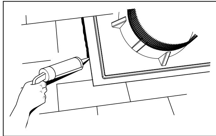
14. Using a good grade of roofing cement material, seal shingles and all screw heads. DO NOT seal the bottom edge of the ventilator base.
