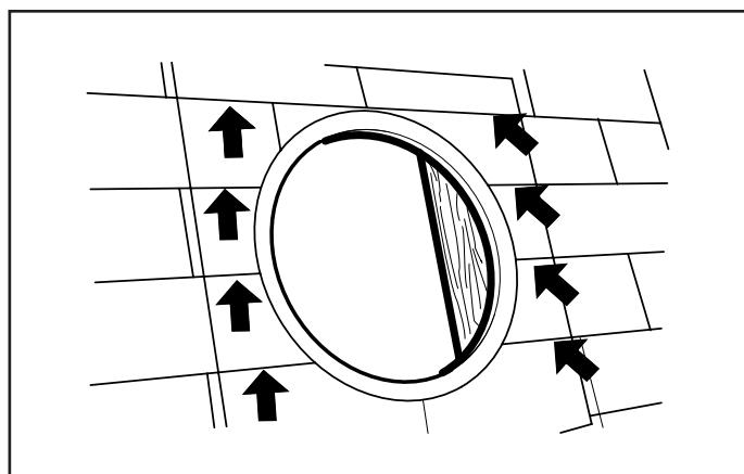
11. For proper removal of roofing nails, draw a 27" square, centered around the hole. Remove nails holding shingles down from top two-thirds of square.
