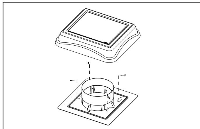
15. Position the ventilator dome so the top points toward the roof ridge. Install the dome to the ventilator base using the four (4) sheet metal screws removed during step 3. Remove cardboard from the solar panel and make sure the ventilator operates.
