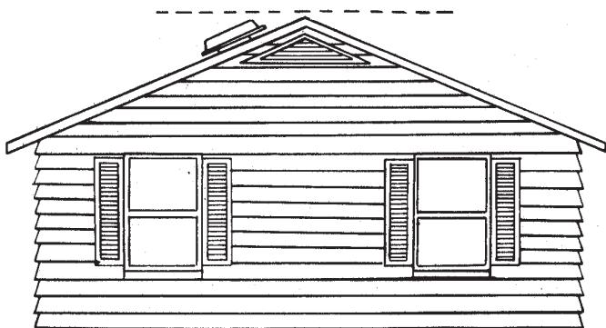
1. Determine the sun's best exposure location on your roof barring shade (trees, other buildings etc.) at 4:00pm in the hottest month of the year. Generally, we recommend a point located 24" – 36" on center below the roof peak and centrally along the ridgeline on the south, southwest, or west side of the home.
