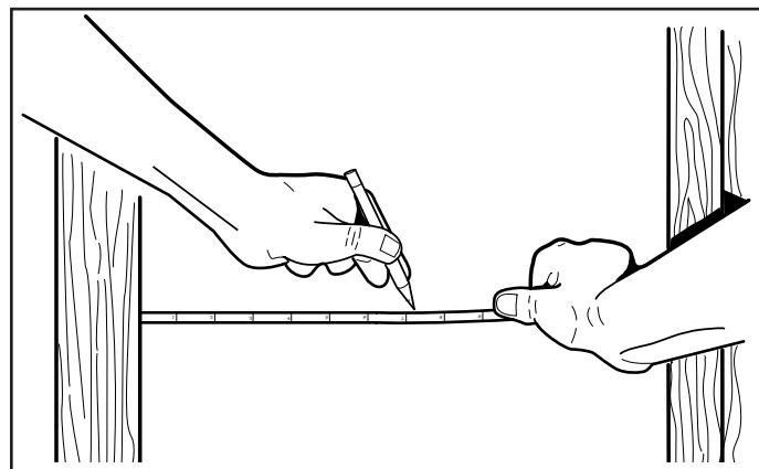
4. Working from the inside of your attic, find the desired ventilator location and mark a spot halfway between rafters at a point that is 24" – 36" below the roof ridge.
