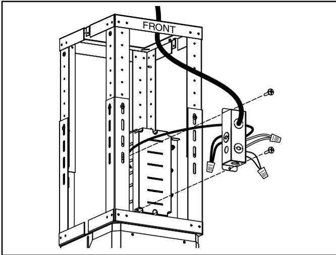
1. Remove wiring cover and connect house wiring to hood wiring – BLACK to BLACK, WHITE to WHITE, GREEN to GREEN. Re-attach wiring cover.
