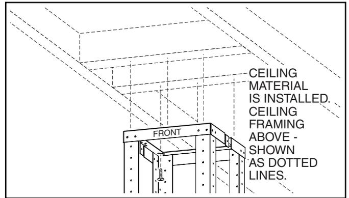
1. Determine length "L" of frame assembly based upon desired installation height (see chart below.) To adjust frame assembly height, remove (8) screws, slide upper frame assembly to required height, replace screws and tighten securely.
